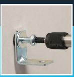
Tighten the screw until the fixing is secure.
